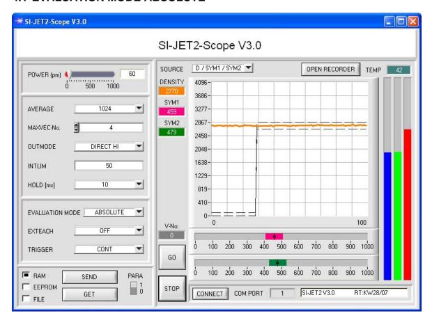
In EVALUATION MODE ABSOLUTE all three channels CH\_L, CH\_C, and CH\_R are used for calculating density, symmetry 1, and symmetry 2:
