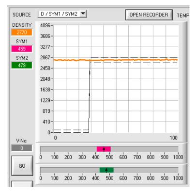
When D / SYM1 / SYM2 is selected under SOURCE, the currently determined values for density, symmetry 1, and symmetry 2 as well as the tolerance windows that were selected under No.: are displayed.
