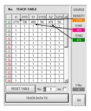
When the GO button is pressed, the DENSITY, SYM!, and SYM2 data that are currently calculated in the sensor are shown on the PC user interface.
